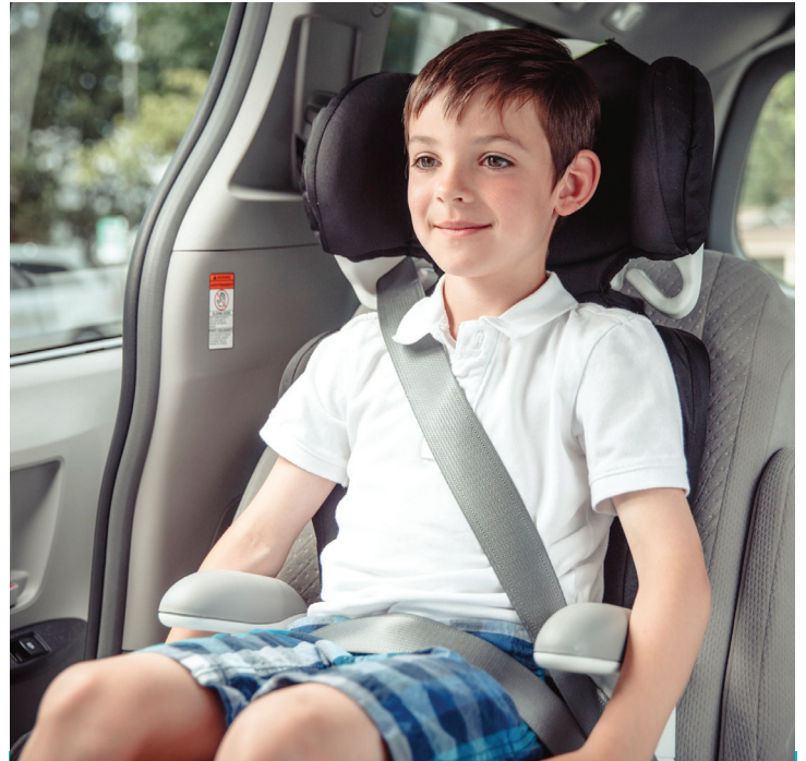
Lap belt is snug across the hips. Shoulder belt lies over the child's shoulder and across the chest.
